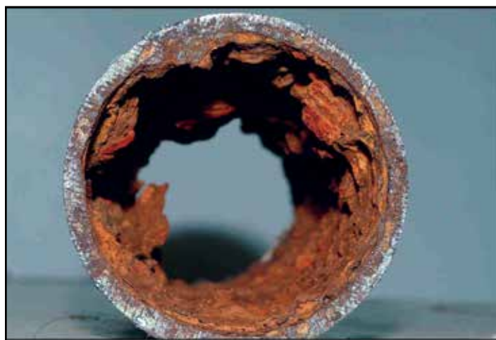
Figure 4. Corrosion product accumulation with subsequent pitting and MIC secondary to low or no flow (top of pipe section appears on the bottom of this photo – note heavier accumulation on the bottom)
